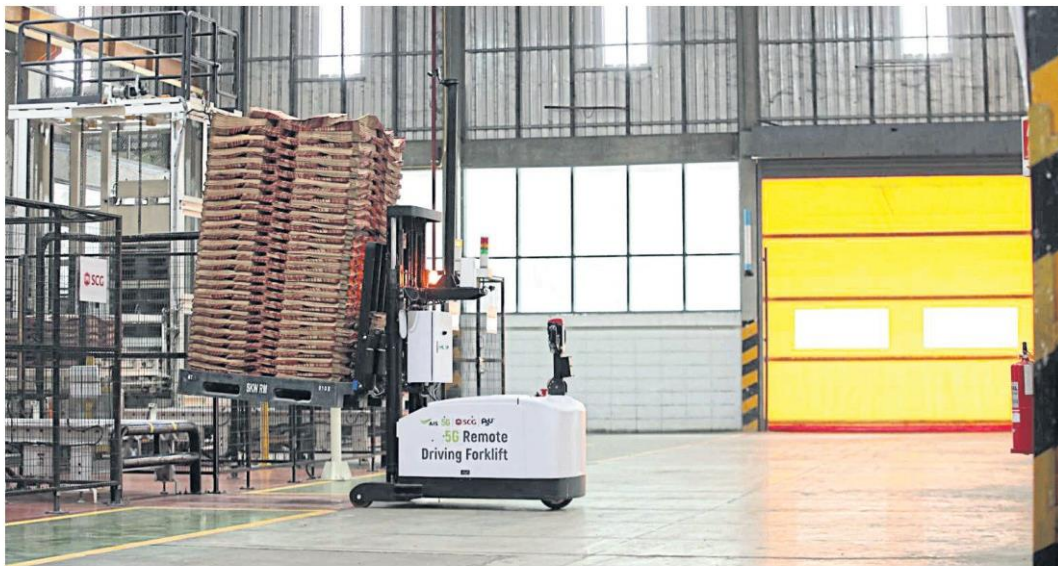
This forklift in Saraburi is remote-controlled from Bangkok using 5G on the 2600MHz range.
