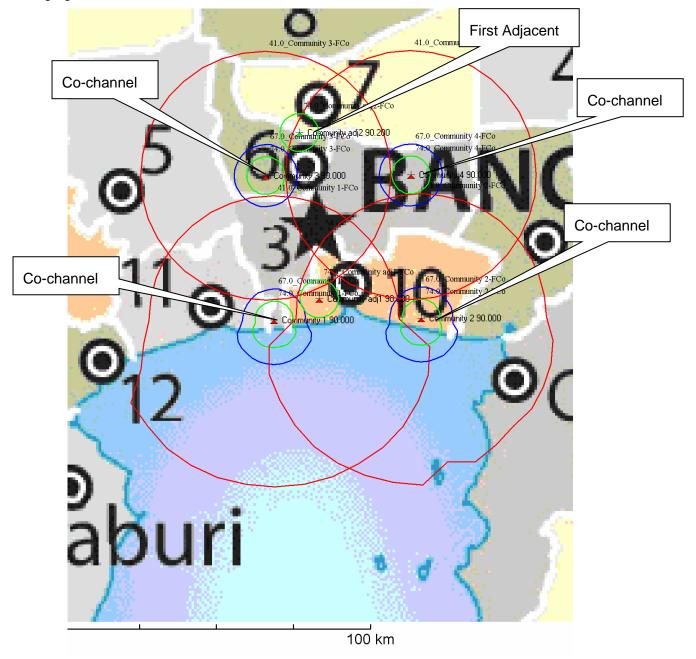
Figure 4: Example of transmitter density for 500W ERP
