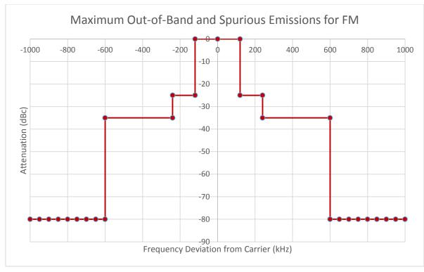
Figure 1: Maximum Out-of-band and Spurious Emission for FAM Transmitters
