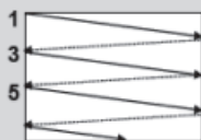
Odd lines in 1st vertical trace.
