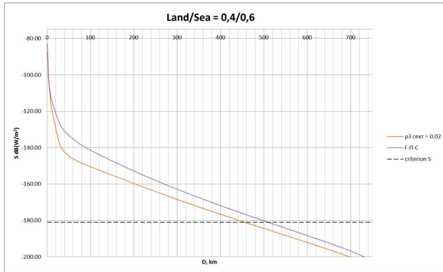
FIGURE 4 Determination of protection distance required in case of IMT stations with 5 MHz bandwidth for mixed path
