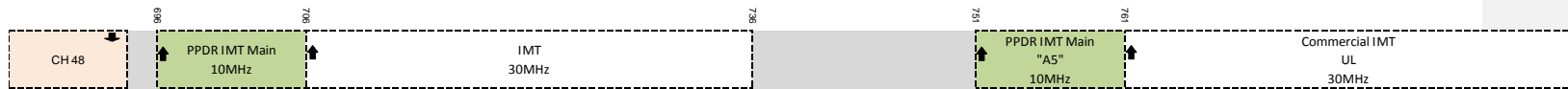
Figure 1. Scenario for PPDR in 700MHz based on UAE proposed arrangement for the 700MHz band of 2x40MHz
