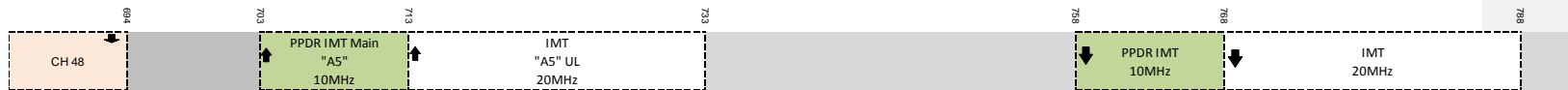
Figure 2. Scenario for PPDR in 700MHz if the Frequency arrangement adopted starts at 703MHz harmonized with APT lower Duplexer
